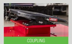
The hydraulic lifting system with Jost coupling ensures that the trailer can be coupled quickly.
