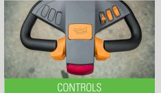
The V-move Trailer Mover is easy to operate with the ergonomic tiller head. Standard equipped with stepless drive control, speed switch and anti-collision protection.
