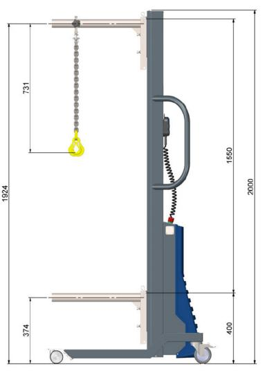
Dimension shown for single arm mounted in reversed position
