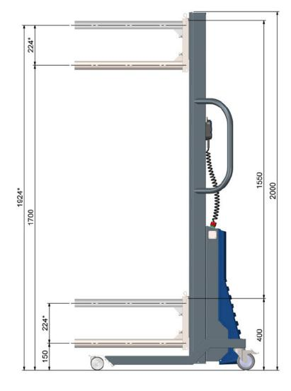
Dimensions marked \* are for the tool in the reversed position
