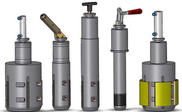
Left to right: 150mm mandrel with pneumatic retract, 75mm toggle retract, 75mm 'T' handle retract, 50mm urethan mandrel with locking toggle handle and 150mm leaf-type mandrel with pneumatic expand and retract.
