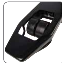
Twin load wheels make it very easy to change direction.
