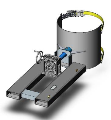
The DSWNH-PBO Sideways Drum Rotator is designed to lift and rotate drums with varying diameters, including standard Plastic Drums as well as barrels - through 360-degree perpendicular to the fork arms. Handle rotation via a Gearbox of the drum cradle ensures minimum effort for fully controlled tipping, allowing complete emptying of the drum contents. Dual woven/chain combination Belly Straps with ratchet tightening for clamping hold the Drum firmly in position.
