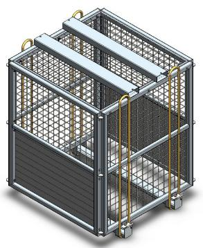
Our MBSN Safety Brick Cages are designed to convey pallets of bricks or similar loose products safely to a work location via overhead crane. Suitable for 1200 mm square pallets (1240 mm clear inside). Signange Panels have been added to two opposite sides outside the mesh paneling.
