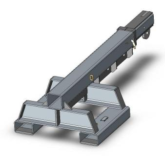
The type MSFJL100 Fixed Jib (Long) is designed as an affordable general purpose Jib with a 3.56 metre reach when fully extended. This Jib has been designed with wide pockets suitable for Forklifts with special hydraulic Tine Positioners. This slip-on Forklift attachment is held to the Forklift by a safety chain. The Jibs overall length when closed is 2.19 metres.
