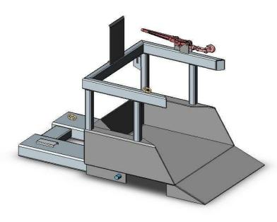
The type MNWBT1 Wheelie Bin Tipper has been designed for emptying a standard 240 litre plastic bin. The Bin is wheeled into the cradle and secured by the Safety Chain attached to the Backrest allowing the bin to be lifted/transported about the workplace and emptied. The tipping operation is simple and safe with the operator never having to leave his seat.
