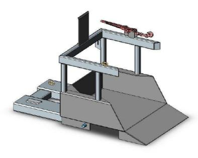
The type MNWBT1 Wheelie Bin Tipper has been designed for emptying a standard 240 litre plastic bin. The Bin is wheeled into the cradle and secured by the Safety Chain attached to the Backrest allowing the bin to be lifted/transported about the workplace and emptied. The tipping operation is simple and safe with the operator never having to leave his seat.
