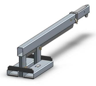
The type MFJL50 Fixed Jib (Long) is designed as an affordable general purpose Jib with a 3.5 metre reach when fully extended. This slip-on Forklift attachment is held to the Forklift by a safety chain. The Jibs overall length when closed is 2.1 metres.
