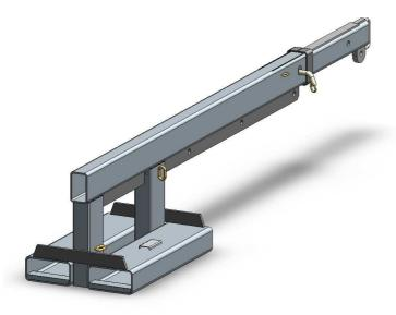
The type MFJL25 Fixed Jib (Long) is designed as an affordable general purpose Jib with a 3.5 metre reach when fully extended. This slip-on Forklift attachment is held to the Forklift by a safety chain. The Jibs overall length when closed is 2.1 metres.
