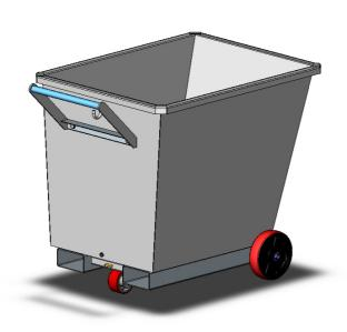
The light weight and cost effective Tipping Fork Skip Bins (type MCFS6 and MCFS9) have been manufactured from 2mm plate and are suitable for goods or waste transport and storage. Fitted with a Forklift carriage and safety chain, two front wheels, a rear swivel wheel and push handle, these Bins are designed for manual push over.
