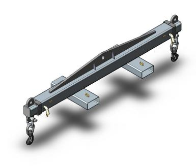
The type MCFM2439 Spreader Beam is a unique multi- tasking Beam which can be used by Crane or Forklift to lift long loads. Using a Crane, loads can be lifted via the centre single hook point (as a ' Lifting Beam'), or end lifted using a 2 leg Chain Sling (as a ' Spreader Beam'). If lifting by forklift, the 600mm long slipper pockets allow for fast and safe connection to the truck.
