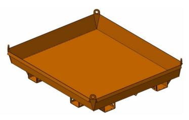
The type MCC110 Concrete Collection Tray has been designed to limit environmental damage wherever a concrete pump is being used on site. This low profile tray fits under the concrete pump to collect spillage washout water and concrete waste. The Tray is fitted with Fork Pockets and Crane Lugs and is manufactured with tapered sides. The overall size of the Tray is 1860 mm x 1560 mm x 360 mm.
