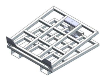
The MBTS10 IBC Container Tilting Stand is designed to effortlessly, and without intervention, allow full discharge of liquid from an intermediate bulk container (IBC). As the volume of liquid contained in the IBC reduces the spring mechanism will raise the rear of the container to an incline up to 10-degrees.
