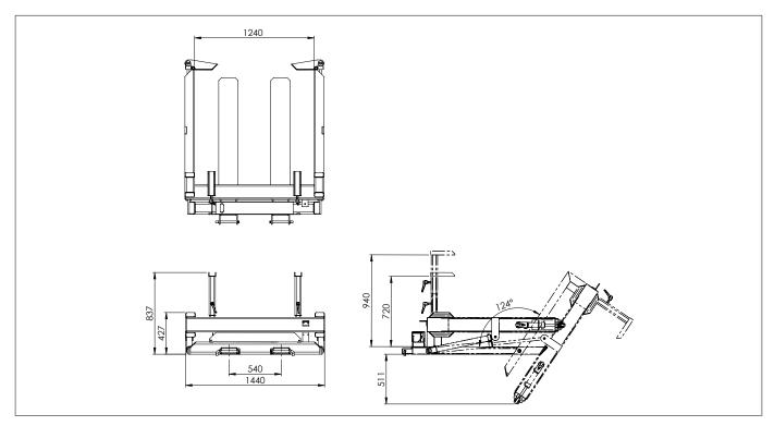
NOTE: MFBTSM requires one hydraulic function. MFBTFH requires two hydraulic function.
