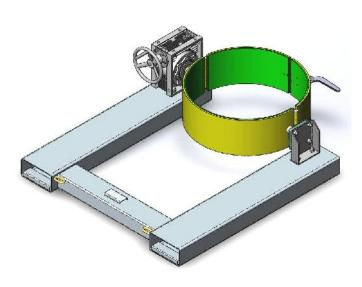
The type DDRNH Drum Rotator is designed to lift and rotate 205 litre Drums through 360-degrees. Handle rotation via a Gearbox, of the drum cradle, ensures minimum effort for fully controlled tipping. This allows a user to empty all the drum contents. A Belly Strap with an eccentric lock holds the Drum firmly in position.
