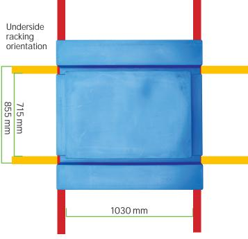
100 x 50 mm bearers required to disperse storage weight to racking (can be supplied).
