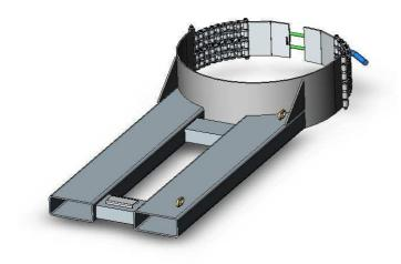
The type DDL1000 Drum Lifter would be considered the safest Drum Lifter available. This unit ensures 205 litre steel Drums are moved with 100% security. The Drum is quickly clamped into the support via the dual Chain Belly Strap & eccentric lock. A further safety catch prevents accidental release.
