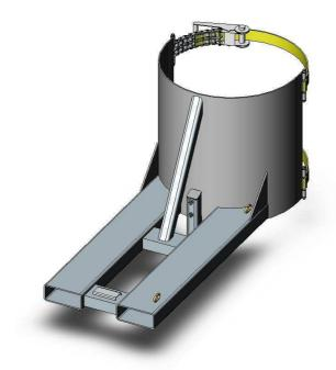
The type DDL1000PBO Drum Lifter would be considered the safest Drum Lifter available. This unit uses dual woven/chain combination belly straps with ratchet tightening to allow clamping of varying diameter drums, including standard plastic drums as well as barrels. With the added feature of a Bin Support Leg, drums/barrels may be moved with 100% security.
