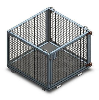
The type MCSPN-01A Crane Goods Cage is designed to convey loose or palleted goods using either a Forklift or Crane. The full width gate allows 1200 mm square pallets to be placed inside the Cage if required.
