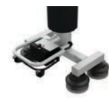
Fixed yoke with 4 bellows suction cups ø75: 190x230, 185x325, 235x325 ø110: 280x370, 330x500 ø150: 350x350
