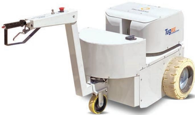
The Tug Rise pedestrian operated electric tug has been designed to tow on slopes or ramps, and is capable of towing up to 1 tonne on a 15 degree ramp with ease, or up to 5 tonne on a flat surface.
