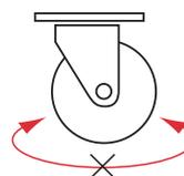
The directional lock tab will prevent the castor from swivelling, by locking it into one position.
