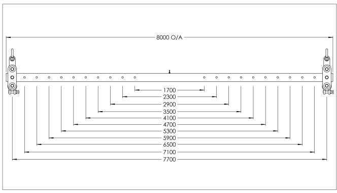
NOTE: The working load limit is calculated on a 60° chain angle setup
