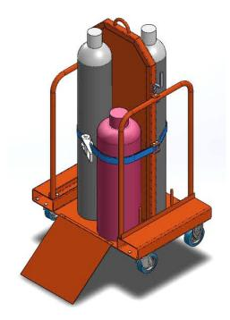
The type MGC4 Gas Bottle Trolley has been designed to suit two type "G" Oxygen and two type "G" Acetylene gas cylinders. Provision has been made to store all hoses inside the cage area. The cage is supplied with internal load binders and straps to securely fasten both sets of cylinders. Fitted with a two point Crane lift, Forklift pockets and 150mm swivel and fixed Casters, this cage can be transported manually, by Forklift or by Crane.
