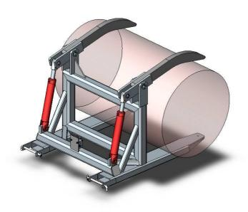
The type MGA-09 Grab Attachment has been designed to grab and secure poles or pipes from 170mm to 900mm in outside diameter and safely lift and transport these by Forklift about the worksite. This slip-on attachment can be fitted in seconds to a forklift requiring only the connection to the 3<sup>rd</sup> function hydraulics, via the quick connect hydraulic couplings, and the installation of two locking pins supplied to prevent the unit from moving off the fork
