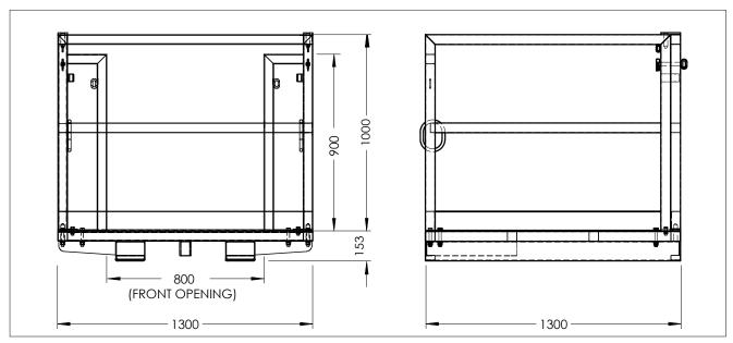
NOTE: Under current Australian regulations outward opening gates are no longer permitted on order picker cages. This cage is manufactured in accordance with Australian Standard AS 5144.3:2019. The load capacity of forklift will restrict the actual load capacity of the Order Picking Cage.
