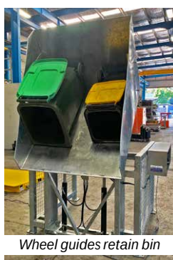
Bin retainers fitted for mega bins
