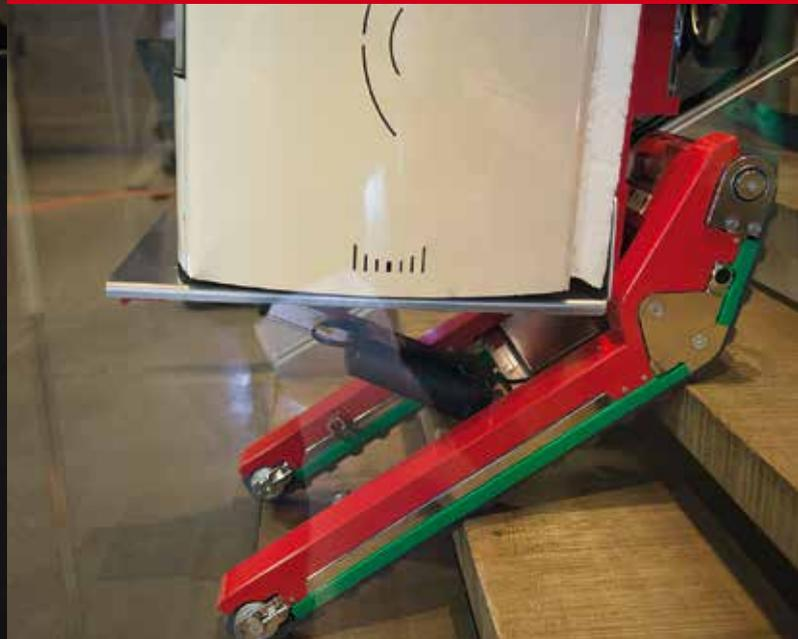
DOMINO is equipped with non-scratching, anti-slip crawler tracks that can rotate 360 degrees. Made of highly resistant special compound, allows you going up and down any type and shape of stairs with ease and safety.
