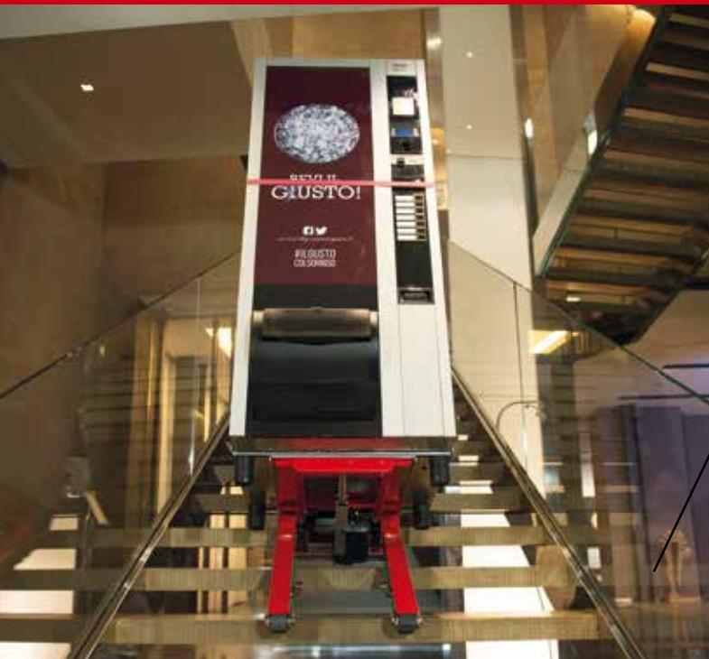
DOMINO Automatic is the perfect partner for bulky and large loads; its independent crawler tracks allow manoeuvring even in narrow spaces, and the weight is always borne by the stair.
