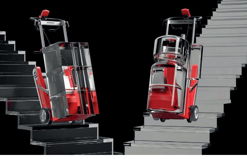
For the transport of heavier and larger loads such as fridges or sofas for example, we recommend using it in "resting on multiple steps" mode as this increases the safety and comfort of travel for the operator, who no longer has to physically manage the load.
