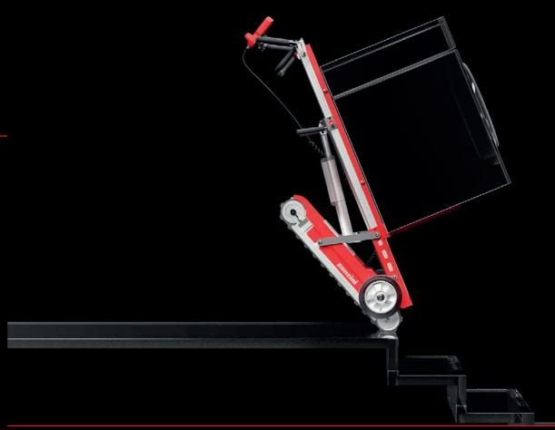
Thanks to the electric piston that controls the crawler tracks, there is no interference between tracks and wheels, therefore entering the landing is extremely easy and stable.
