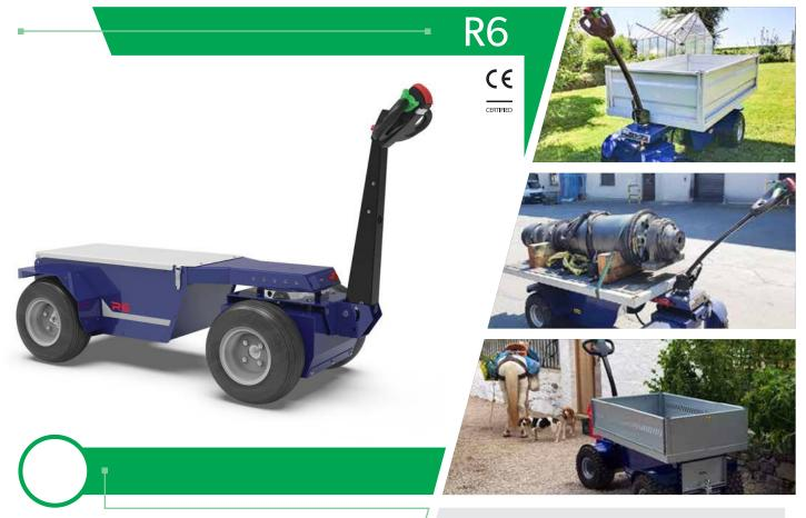
**Zallys R6** is a 4 wheel off road tow tug that has been designed to be used on difficult grounds like sand or mud. It is equipped with 2 motors. It's been designed to load up to 800 kg on flat grounds and has a towing capacity of up to 6000 kg.
