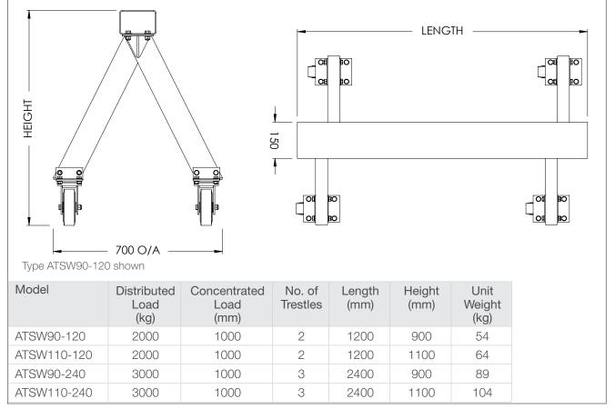
NOTE: Optional ATR120 Rubber profile channels are supplied in 1.2m lengths. 2 units required for 2.4m long trestles
