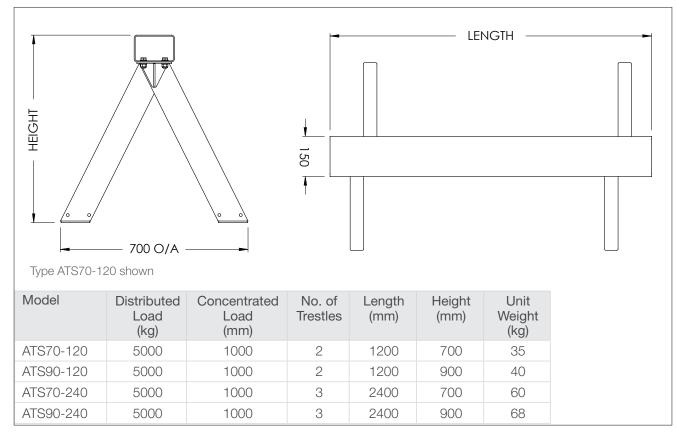
NOTE: Optional ATR120 Rubber profile channels are supplied in 1.2m lengths. 2 units required for 2.4m long trestles
