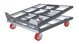
MBTS10-W IBC Bin Tilter with wheels is designed to effortlessly and without intervention allow full discharge of liquid from an intermediate bulk container (IBC). As the volume of liquid contained in the IBC reduces the spring mechanism will raise the rear of the container to an incline of up to 10 degrees. Fitment of one spring is suitable for most applications. For heavier metal construction IBC's, the unit can be easily adjusted to suit the load weight by simply adding additional springs.
