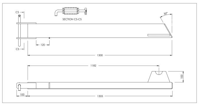
NOTE: This unit is made to order and non returnable. Please ensure fork tines are measured to ensure correct fit. The MDCS1 suits a maximum 100x45mm fork size. For fork sizes above this (even if you have a 2.5T forklift), you must order the next size up. For example a 2.5T Forklift fitted with 125x45mm fork size suits the MDCS2.
