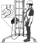
Ascend ladder to desired position. Use work positioning hook to attach
