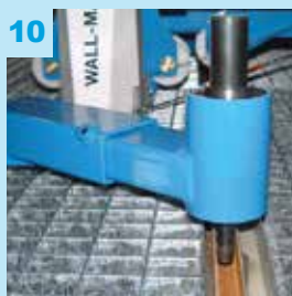
Floor guidance of lower support wheels.
