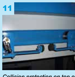
Collision protection on top of mast when more than one WALL-MAN® on same rail.
