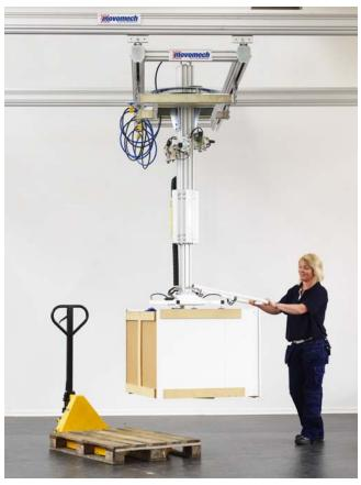
The lifter is so constructed that it can be fitted with standard or specially constructed tooling and with accessories such as a rotation unit, different tooling fixtures, braking unit etc. This allows the Mechlift to be easy adaptable for different applications and for lifting and handling within many different branches and sectors. The lifter is built upon telescopic operating profiles in aliuminium that are anodized which are thereby complete free from maintenance.
