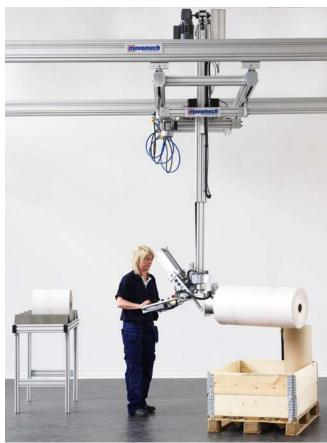
The Mechlift – Electric is an ergonomically designed moment absorbing lifter that has a stepless frequency steered lifting speed that is controlled via joystick.
