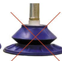
Insufficient vacuum level
