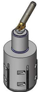
"Rotating Mandrel" (mandrel rotates to allow material winding)
