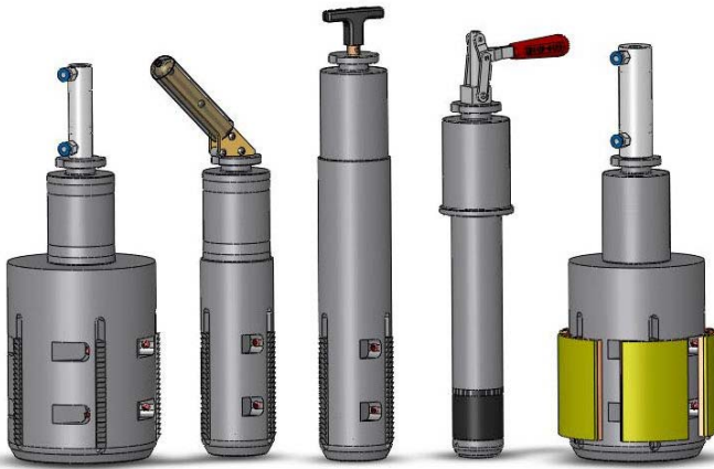
Left to right: 6" mandrel with pneumatic retract, 3" toggle retract, 3" "T" handle retract, 50 mm urethane mandrel with locking toggle handle and 6" leaf-type mandrel with pneumatic expand and retract.
