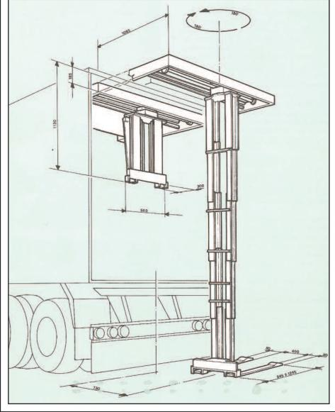
It can be installed on the top inner side of the van and thanks to its reduced overall dimensions; it enables the complete loading of the vehicle even on two stages, still having the possibility of placing the pallets in their best position.
